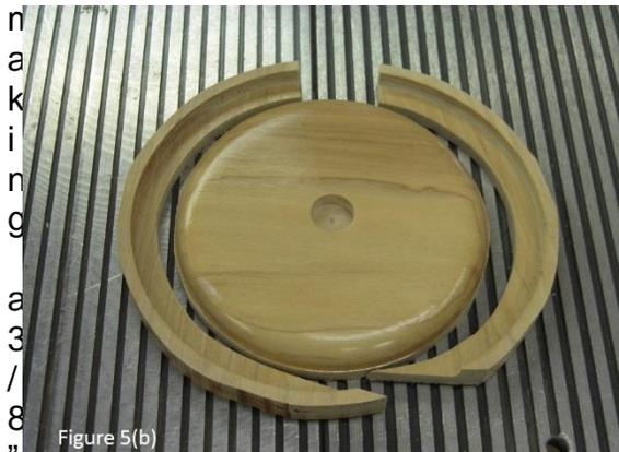
groove around the line. Cut the groove about  $1/2$ " deep, this will provide tool space for shaping the lid's outside edge. Shape the lid top and edge, Figure 5(a). Drill a  $3/4$ " diameter hole,  $3/8$ " deep, for the pull. Sand top of lid to 320 grit and finish. Remove the lid from Jumbo Jaws, use bandsaw to separate the groove from the lid, Figure 5(b).
